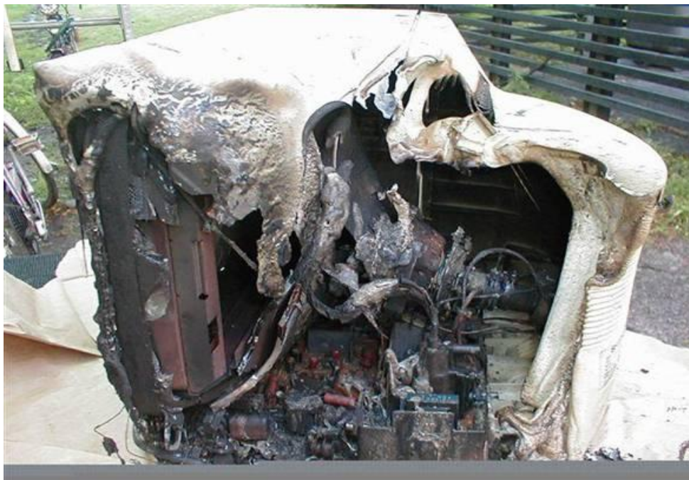
Figure 3: TV set destroyed by fire
