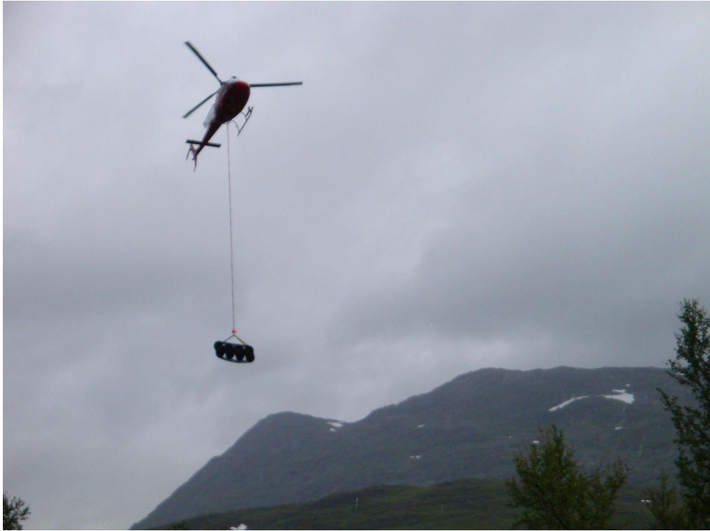
Figure 2. Helicopter transport of Crawler Drilling Machine.
