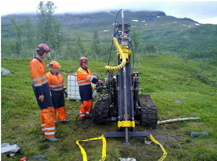
Figure 1 (a). Crawler Drilling Machine
