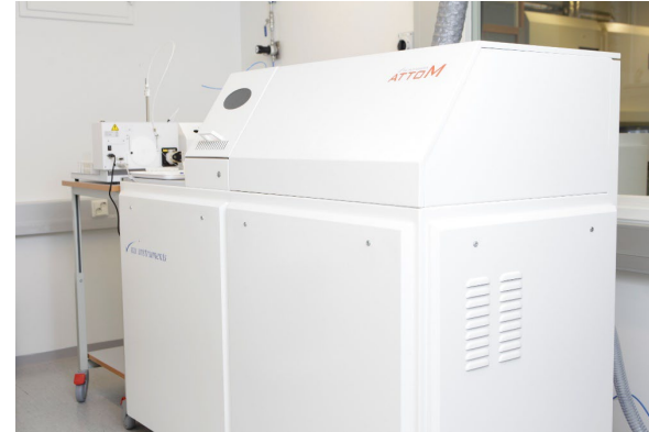
LA-SC-ICPMS for trace elements
