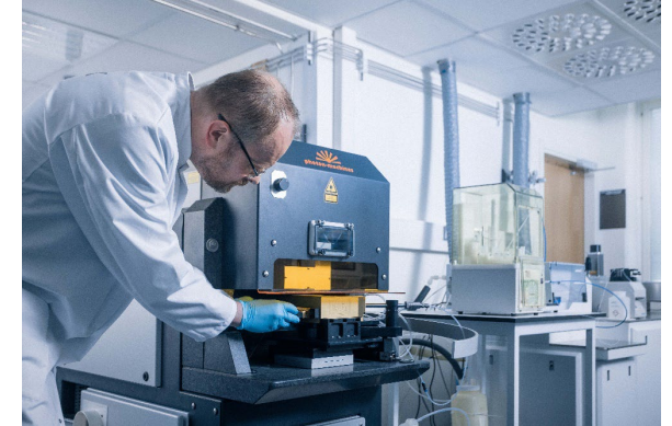
LA-SC-ICPMS for trace elements
