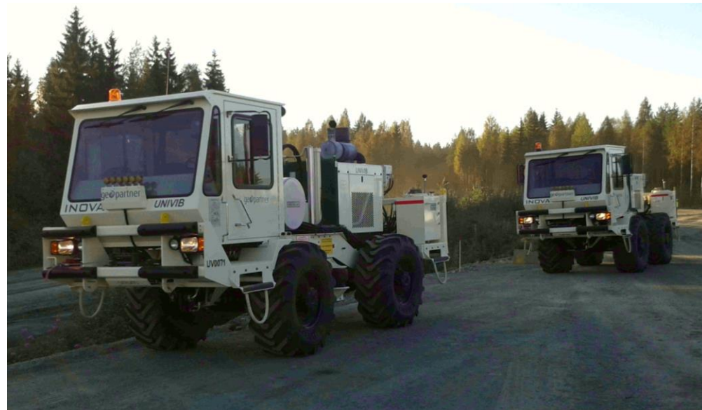
Seismic source in action
