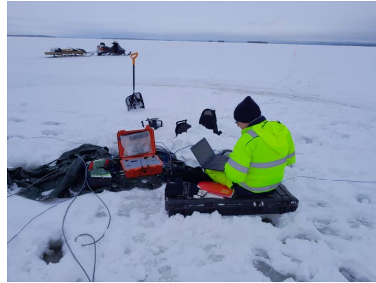
Installation of a magnetotelluric sensor on frozen lake
