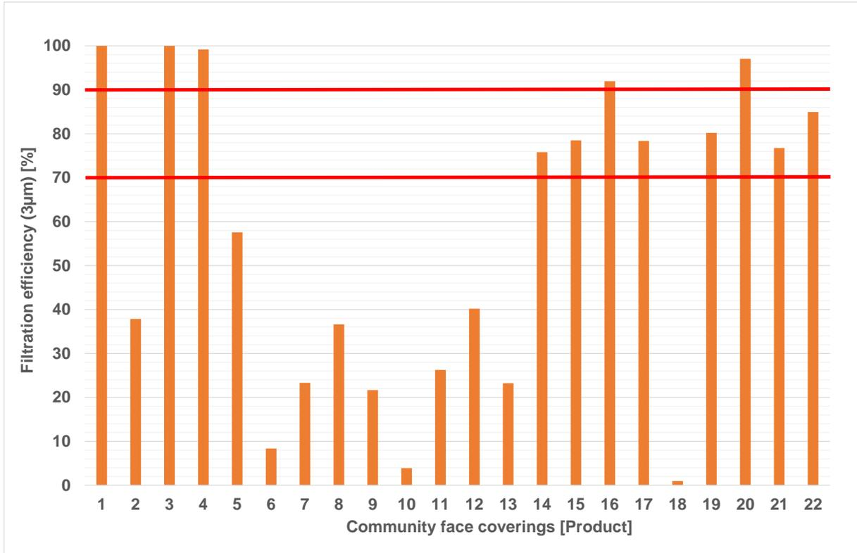
Figure 3. The filtration efficiency of the community face coverings (average, particle size 3 µm).
