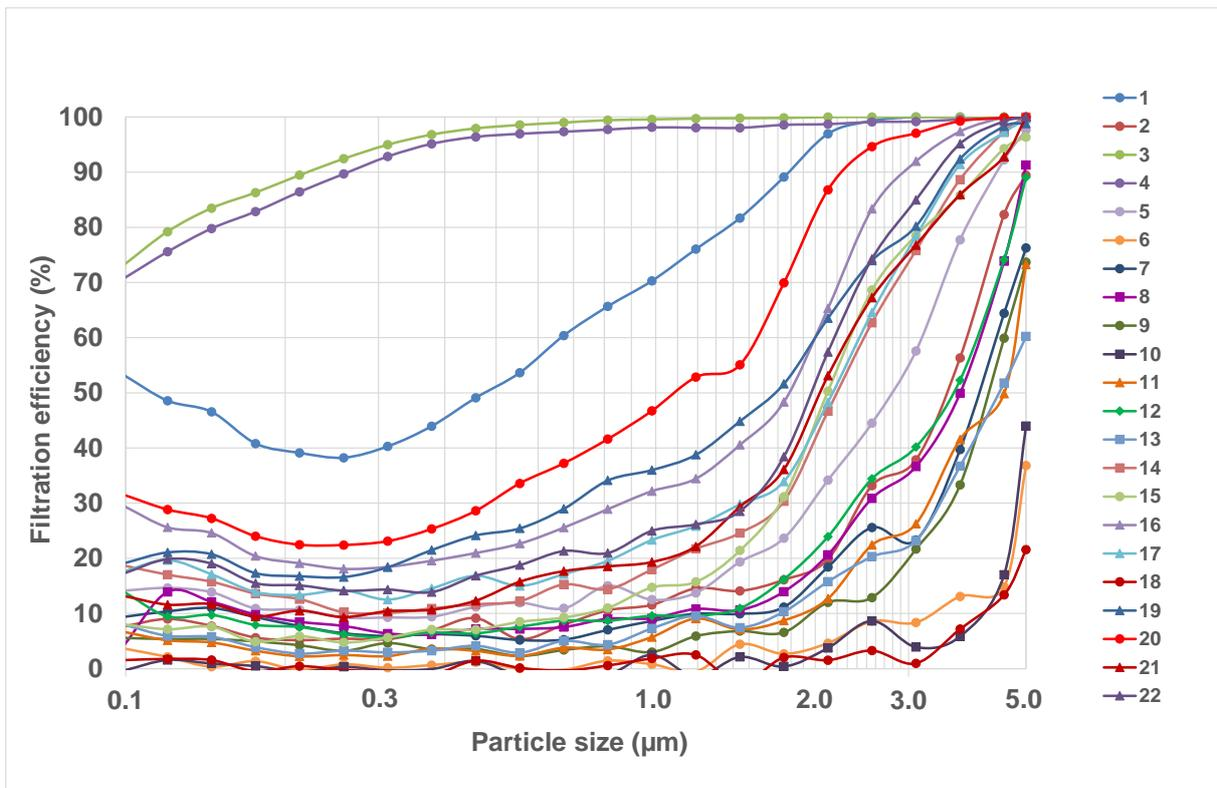
Figure 4. The filtration efficiency as a function of the particle size range of the community face coverings.
