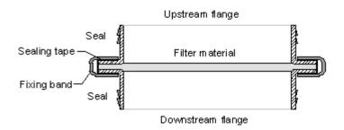
Figure 1. Principle of the sample adapter.
