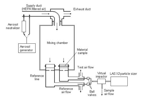
Figure 2. Principle of the test system.
