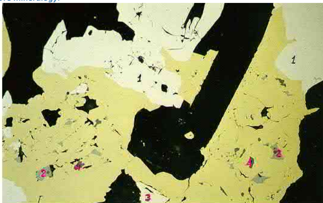
Ängesneva. Gudmundite (1), tetrahedrite (2), pyrite (3), and sphalerite (4) as inclusions in chalcopyrite. Field of view 0.4 mm. From Kojonen et al. (1991).
