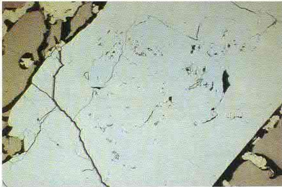
Euhedral arsenopyrite, with loellingite core and inclusions of aurostibite, Bi telluride, native bismuth and Au telluride, in pyrite-pyrrhotite matrix. Field of view 1.17 mm. From Kojonen et al. (1991).
