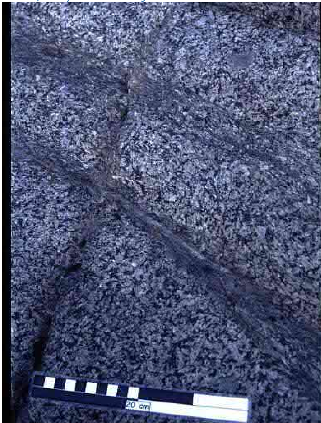
A set of narrow, arsenopyrite- and gold-bearing shear zones, and a post-gold fracture with reddish retrograde alteration envelope at Vesiperä. Photo Pasi Eilu 1/10/1997.
