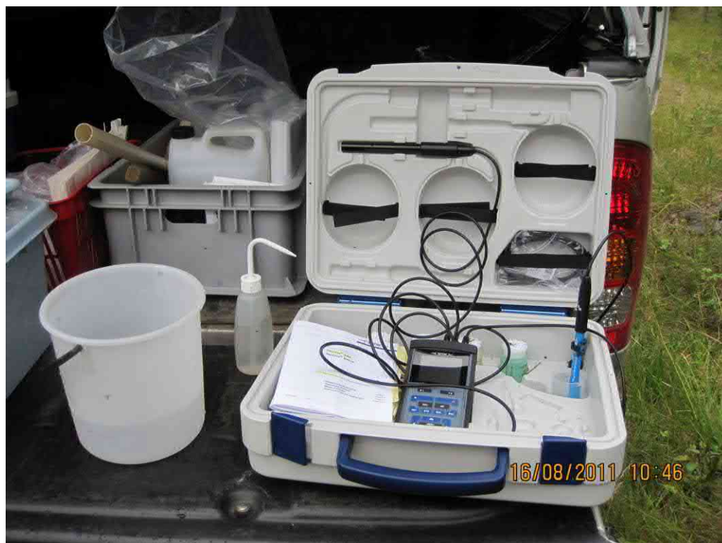
Fig. 7. Multiliner meter for field measurements of waters (WTW Multi 3430 SET F).
