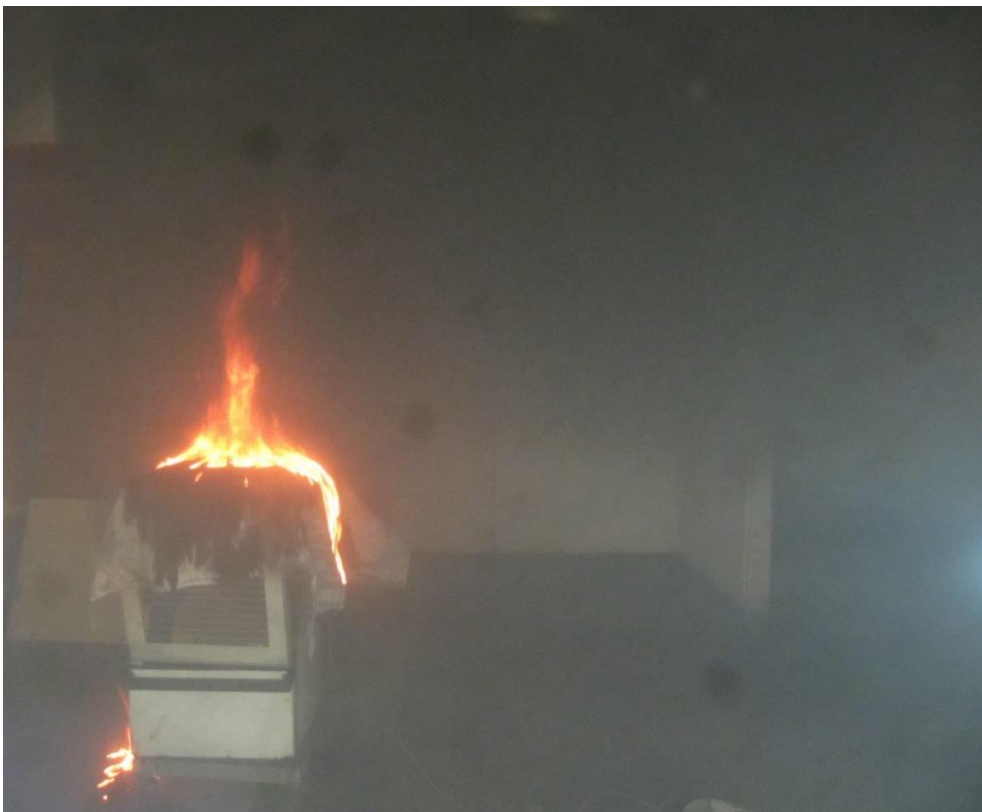
Figure 9. Test room in the fire theatre during the polyurethane fire
