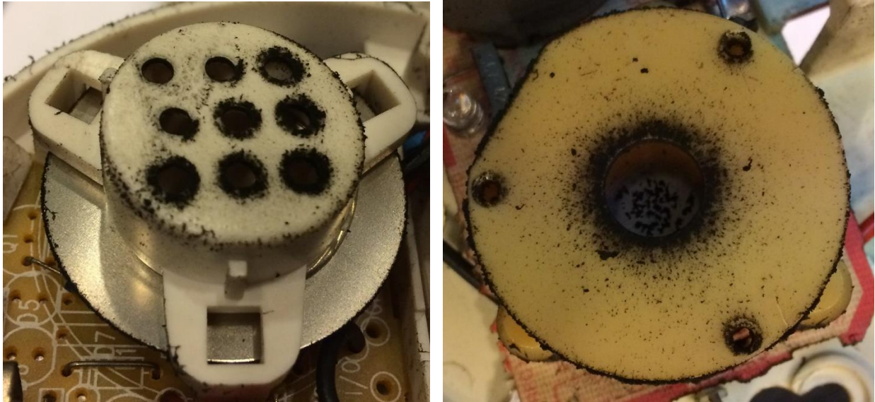
Figure 10. Dirt near the buzzer after testing
