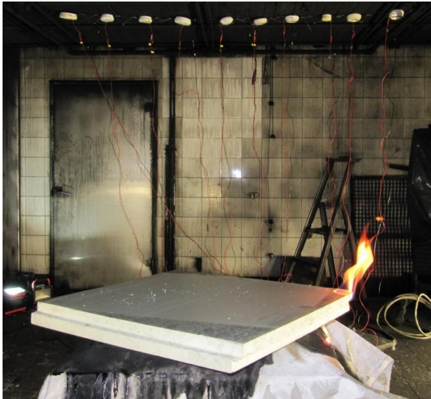
Figure 8. Polyurethane board after ignition
